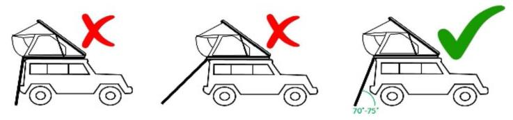
The ladder may need to be adjusted to achieve the correct angle depending on the height of your setup. If shortening is required, the adjustment must be done from the top. Ensure the ladder is fully extended and all rungs are locked in place. Press the first set of locking buttons (second rung from the top) and allow the ladder to compress until a gap of approx. 3.3 inches is achieved between rung 1 & 2.
