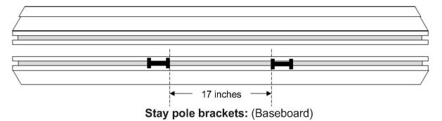
These are to be fitted at the rear 4.33 inches in from the corners of the bottom baseboard.
