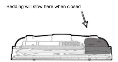
**NOTE:** The amount of bedding left in tent may affect closure. If tent is not folding and closing smoothly, bedding may be too bulky and must be removed. Forcing closure may put undue pressure on components and cause failure which will not be covered by warranty.
