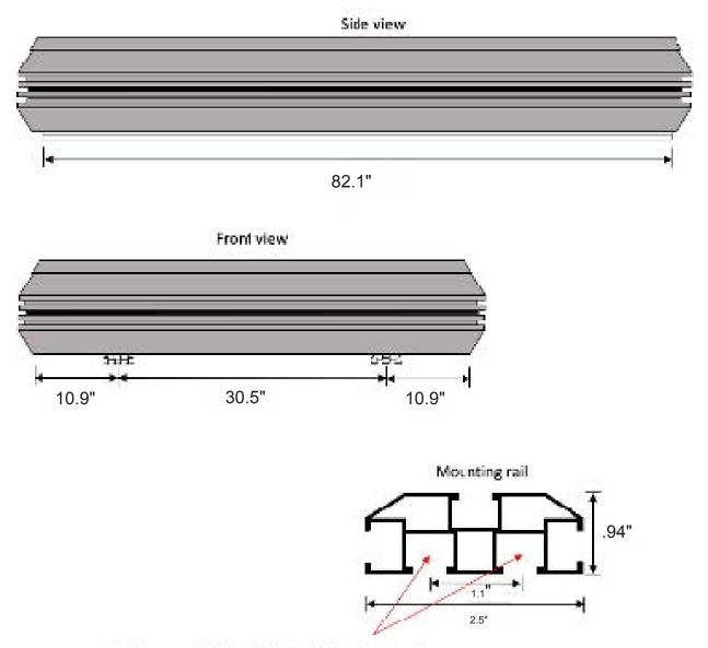
Slide mounting bolt in to either channel.
