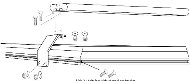
Slide 2 x bolts into slide channel per bracket
