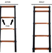
If further shortening is required press the second set of locking buttons (third rung from the top). This will close the 85mm gap until rung 1 & 2 are now touching. Swing in the bottom of the ladder until it supports the weight of the roof top tent. If the angle of the ladder is between 70° and 75°, this adjustment is complete.
