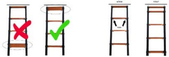
If further shortening is required press the second set of locking buttons (third rung from the top). This will close the 85mm gap until rung 1 & 2 are now touching. Swing in the bottom of the ladder until it supports the weight of the roof top tent. If the angle of the ladder is between 70° and 75°, this adjustment is complete.
