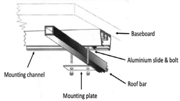
Inspect the position of the roof top tent to ensure it will open in the desired position. Place a mounting plate under the roof bar whilst locating the bolts and hand tighten lock nut. Repeat for all 4 corners. Double check the tent's position as desired and tighten all nuts securely with 13mm wrench. Insert end caps into the ends of the mounting rails, this may require light taps with a hammer.
