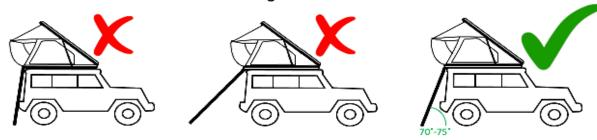
The ladder may need to be adjusted to achieve the correct angle depending on the height of your setup. If shortening is required, the adjustment must be done from the top.
