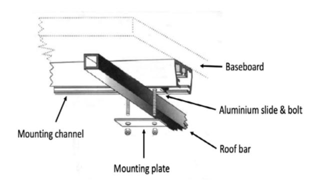
**Note:** It is recommended the rear of the tent is flush with the back of the vehicle to allow correct ladder angle. Place a mounting plate under the roof bar whilst locating the bolts, insert washer and hand tighten lock nut. Repeat for all 4 corners. Double check the tent's position as desired and tighten all nuts securely with 13mm wrench. Insert end caps into the ends of the mounting rails, this may require light taps from a hammer.
