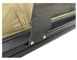
4. Using a 5mm Allen key, tighten the bolts.
