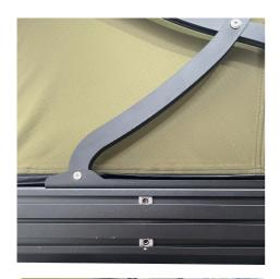
1. Slide in two of the channel nuts. One in the top channel, one in the lower in desired awning bracket position. Optional: Slide an additional channel nut in the underside channel.
