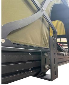
2. Align your bracket with the channel nuts and insert the washer first, then the M8 bolts in line with the nuts
